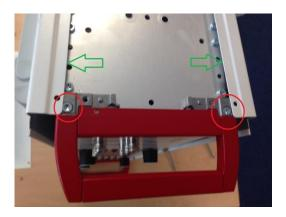
3. Remove the marked screw(s) (not all visible in photo), which are not necessary for the stability of the DLC pro's assembly.
