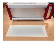
2. Remove the top and bottom plate (push in the direction indicated by the green arrows). Remove the handle (unscrew the screws marked with a red circle).
